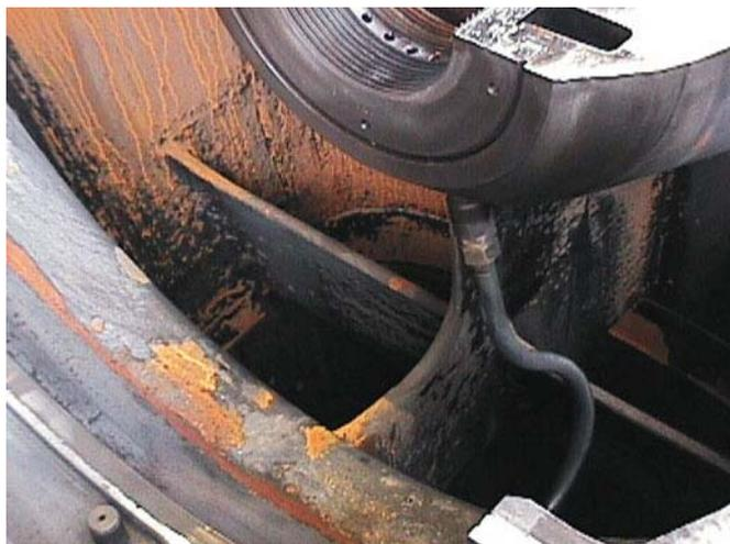
Figure 1: First Condensate Corrosion: Damage to a Turbine.
